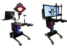
Two cart system examples, one LCD Monitor and one ColorDome on an operating room (OR) cart for testing supine or seated patients
