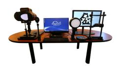
An example of a desktop system with 4 stimulators: the ColorDome, ColorFlash, Envoy, and LCD Monitor provide a complete testing suite
