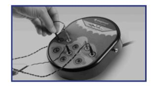
**Ultra-Sensitive Amplifier** A fully differential, high-resolution 1 nanoVolt (nV), 32-bit amplifier with a 5 volt range and common mode rejection
